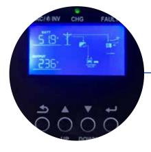
Graphic LCD display with all relevant information on operating mode, input and output voltage, frequency, output power and battery charge level
