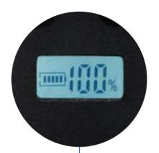
Charge status display via LCD display
