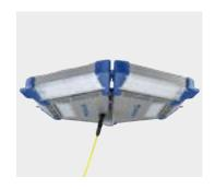
Aluminium / plastic housing, clear polycarbonate cover with lens optics, detachable power supply cable with mains plug and potentiometer, infinitely adjustable, incl. adapter for spigot (DIN 14640 certified) with the possibility of straight or 30° angled assembly, incl. transport cover.
